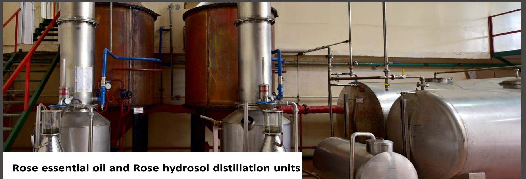
Extracting Rose essential oil and Rose hydrosol
